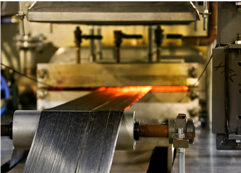
Heating of precursor materials into carbon fibers (Courtesy of the Oak Ridge National Laboratory / DOE)
